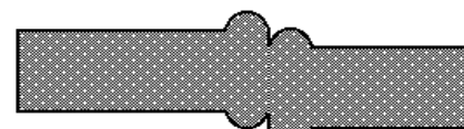
6. Disallineamento, tolleranza massima consentita 10% dello spessore della parete del tubo Disalignment, tolerance accepted 10% of pipe wall thickness
